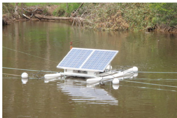
Figure 4.28 Solar water circulation system close up
