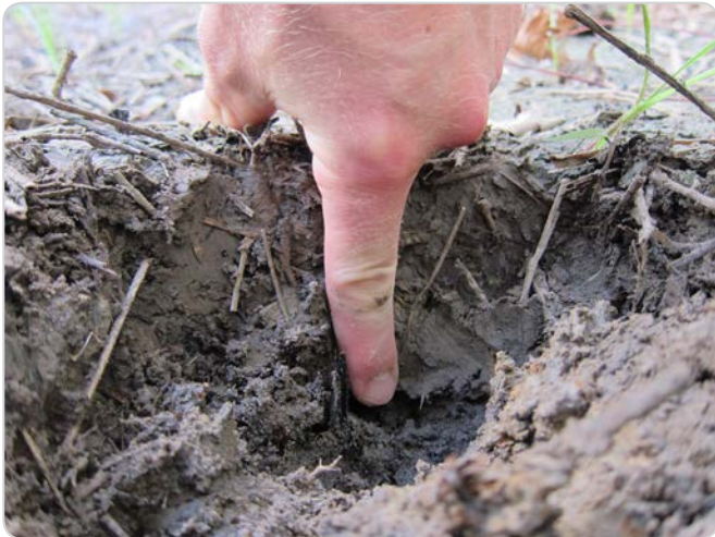
Figure 42: Sediment accumulation on the system's surface
