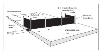
Typical sediment fence installation detail showing 'returns'. (Source: Catchments and Creeks Pty Ltd)
