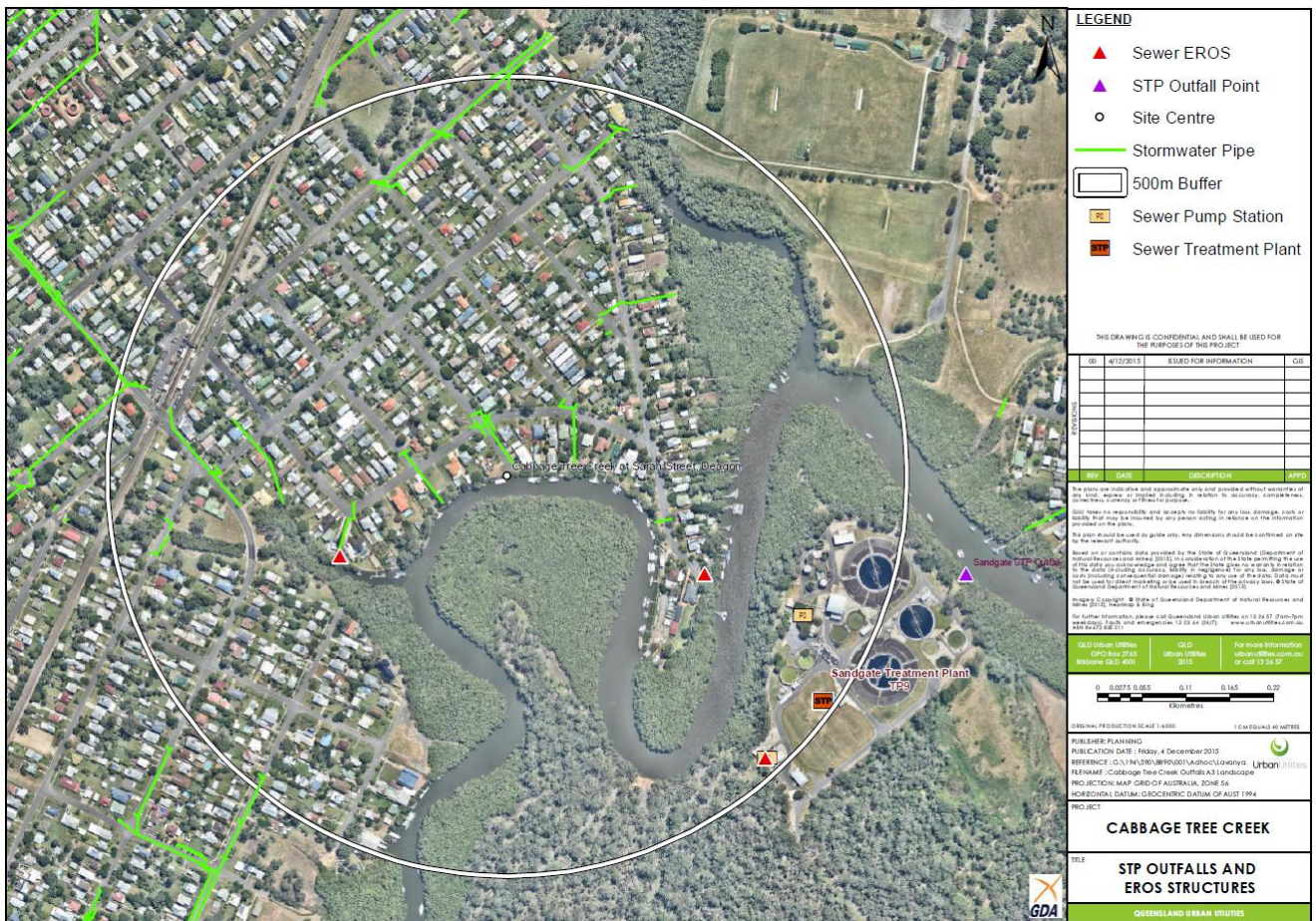
Figure 6: Sewerage infrastructure, including EROS and potential stormwater transport pipes within 500 m of a recreational water site. Recreational site is white dot in the centre of the 500 m perimeter.
