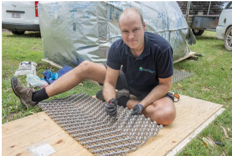
Bureau Waardenburg's Wouter Lenjkeek prepares the potato starch artificial reef he helped develop.
