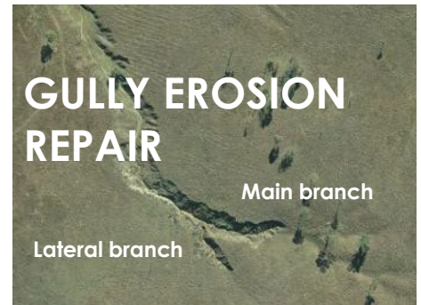
Aerial image showing main and lateral branches of an active eroding gully.
