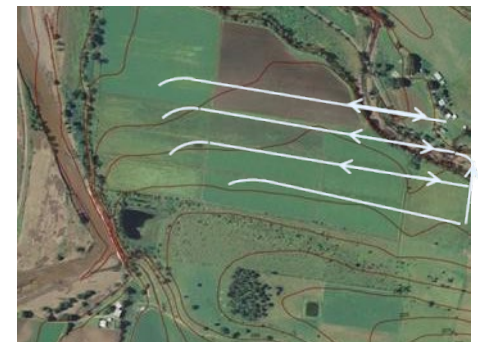
A well designed drainage plan manages the volume and velocity of runoff and safely conducts it to stable discharge points.
