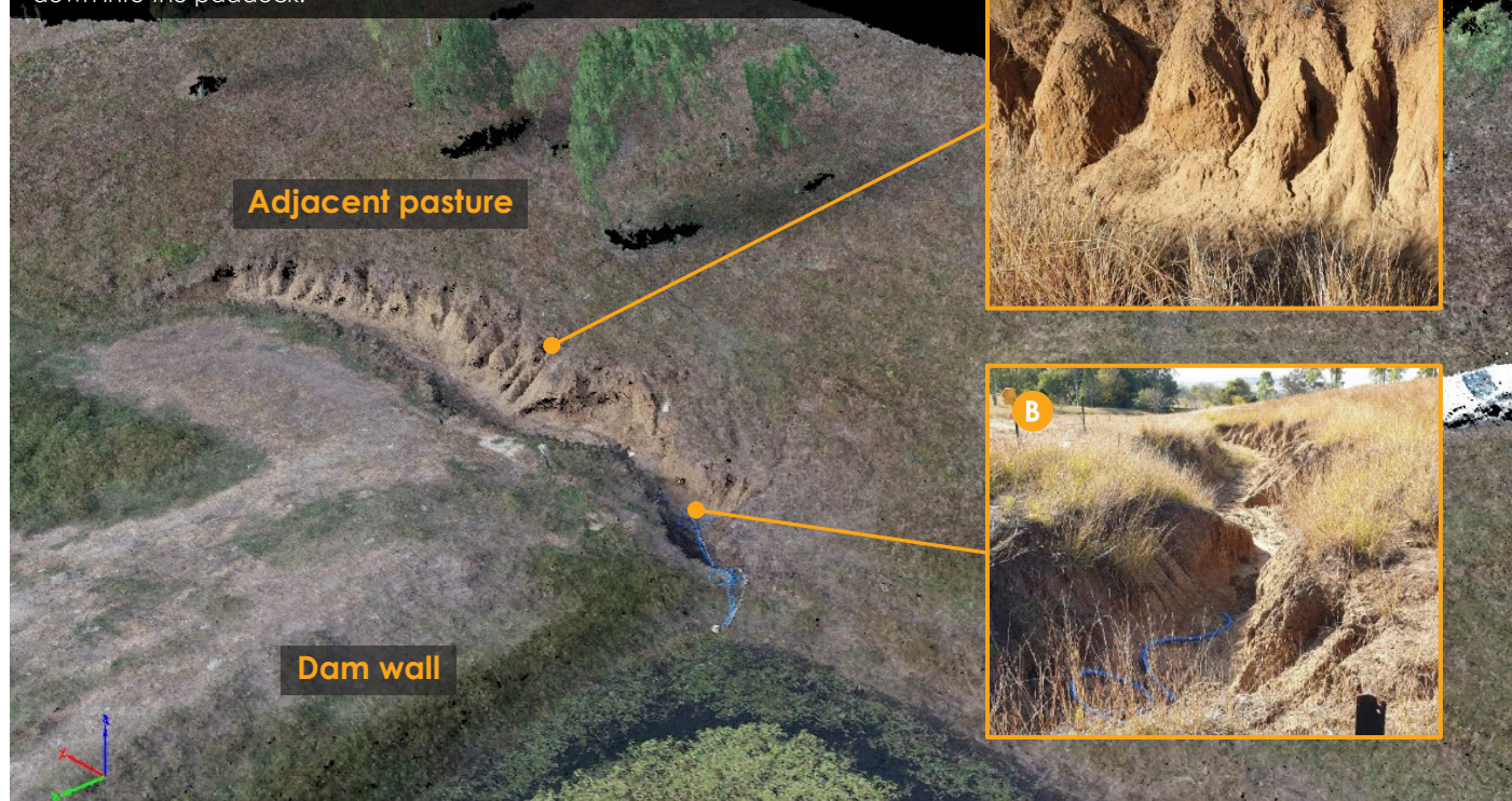
Figure 2. Aerial view of the erosion site before the erosion control work began. Inset A shows where runoff from the adjacent pasture was causing further damage. Inset B shows where the gully erosion continued from the dam wall down into the paddock.
