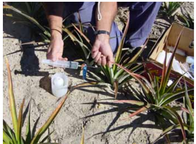
Field testing soil nitrogen levels using Mottes tubes.
