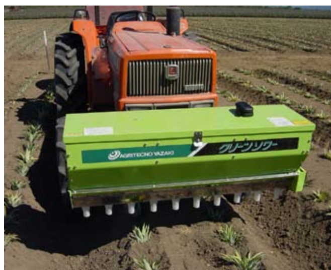
Pineforce Pty Ltd have had great success using the Agritechno Yazaki seeder to sow living mulch in their inter-rows. The seeder is designed for easy fitting and removal.
