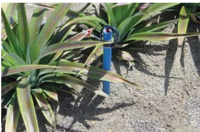
Two sizes of Mottes tubes were used to collect soil-water solution.
