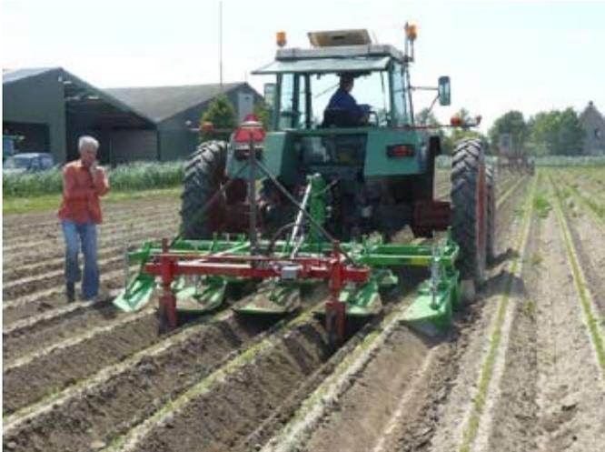
Figure 2. Tractor on 3.15 m track width with guidance on both the tractor and the implement. (BioTrio Farm, The Netherlands)
