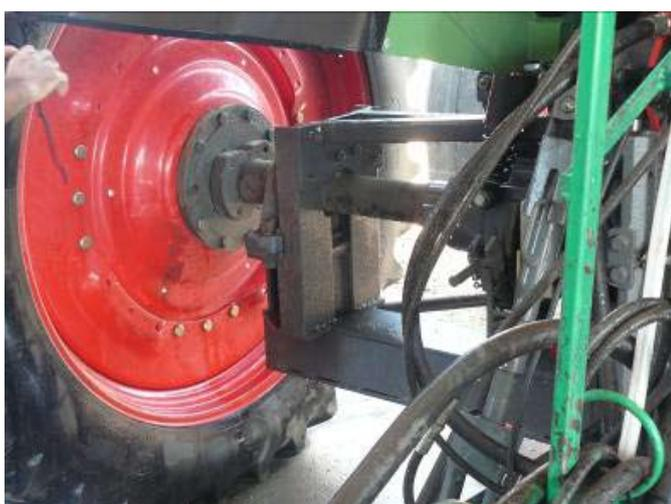
Fig. 3. New front axle, cotton reel and rear axle modifications to provide 3.2 m track width on tractors (Kjeldahl Farm, Samsø, Denmark)
